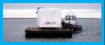
A tugboat carefully guides a barge containing components of the Arviat Research Support Centre. The Igloolik, Cambridge Bay and Rankin Inlet facilities were also shipped by sealift.
