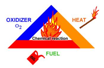
Fire will not be initiated if any one of these elements is absent, and will not be sustained if one of these elements is removed. This concept is useful in understanding prevention and control of fires. For example, the coexistence of flammable vapours and ignition sources should be avoided, but when flammable vapours cannot be controlled elimination of ignition sources is essential.
